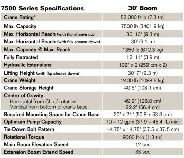
\*Crane rating (ft-lb) is the rated load (lb) x the respective distance (ft) from centerline of rotation with all extensions retracted and lower boom in horizontal position.
